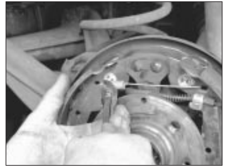
6.5a Unhook the upper return spring from the front shoe . . .
