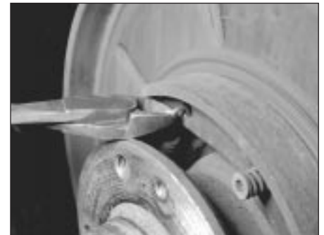
12.7b Remove the upper shoe return spring
