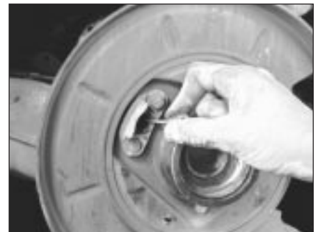
10.6 Pull the cable out of its conduit; before you refit the new cable, be sure to lubricate it with multi-purpose grease
