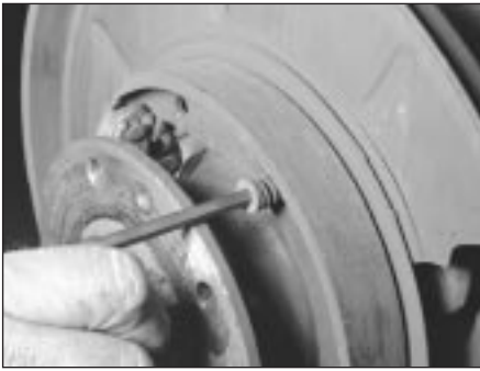
12.7c Remove the shoe hold-down springs
