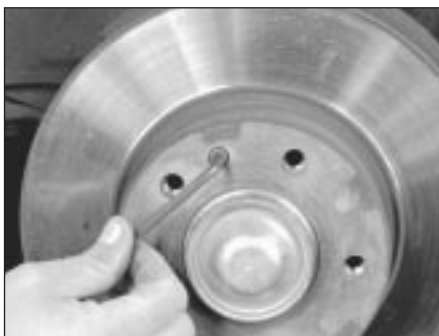
5.6a Remove the disc retaining screw . . .
