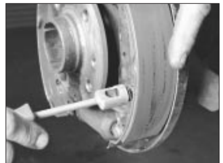
6.6b . . . and the rear shoe hold-down spring
