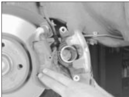
3.5d Remove the caliper, brake pad wear sensor and inner pad all at the same time (3-Series), then refit the inner pad on the piston and press the piston fully into the bore with a C-clamp
