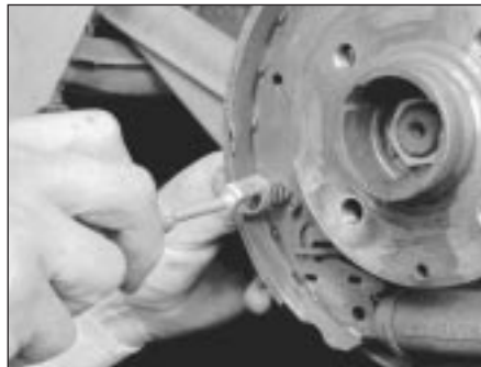
6.6a Remove the front shoe hold-down spring . . .
