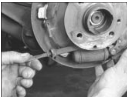
6.8 Remove the automatic adjuster assembly
