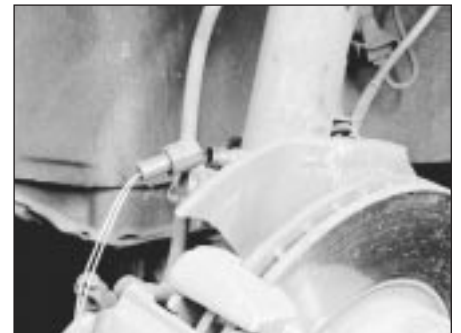
3.5f On 5-Series models, unplug the electrical connector for the brake pad wear sensor
