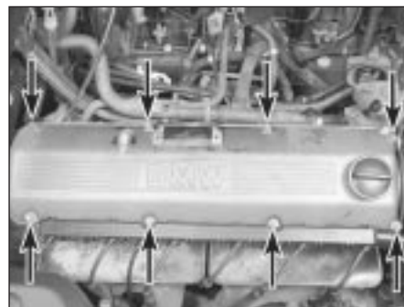
4.6b Valve cover bolt locations (arrowed) on M20 six-cylinder engines
