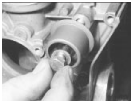
14.11a Removing the stabilising roller from the front end cover (M40 engine)
