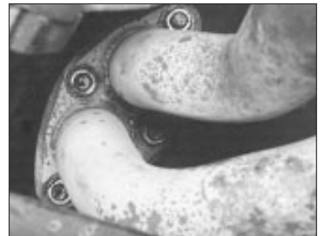
6.5b Exhaust manifold-to-downpipe flange (M40 engine)
