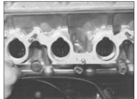
5.15b Removing the lower intake manifold gasket (M40 engine)
