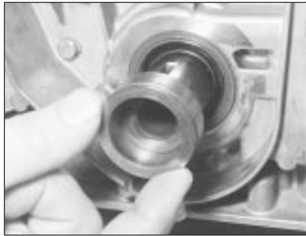
14.13 Removing the spacer ring from the front of the crankshaft
