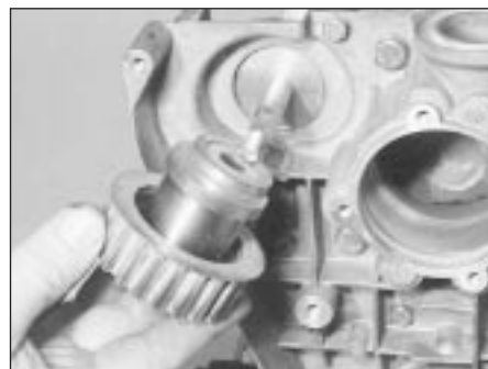
14.8 Removing the timing belt tensioner (M40 engine)
