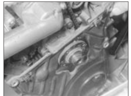
9.9c Removing the lower timing belt cover on the M40 engine
