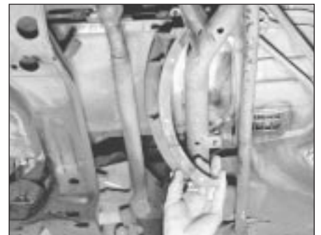
13.6b . . . remove the cover to get to all the sump bolts
