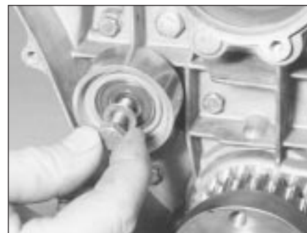
14.11b Removing the guide roller from the front end cover (M40 engine)
