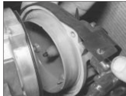
9.6a Unbolt the distributor cap (M40 engine) . . .
