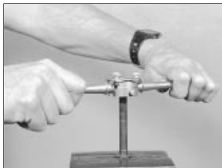
12.25 A die should be used to remove sealant and corrosion from the head bolt threads prior to installation
