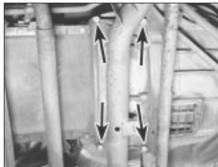
13.6a Remove the four inspection cover bolts (arrowed) and . . .
