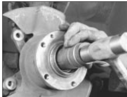
8.10 Use a large socket or a suitable piece of pipe to drive against the inner race of the new bearing
