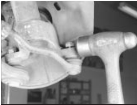
17.2 Loosen the nut on the track rod balljoint stud. For preference use a balljoint separator; otherwise, give the steering arm a few light blows with a hammer to release the balljoint stud. Remove the nut, and separate the balljoint stud from the steering arm
