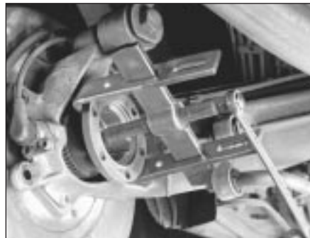
15.11 Remove the drive flange with a puller
