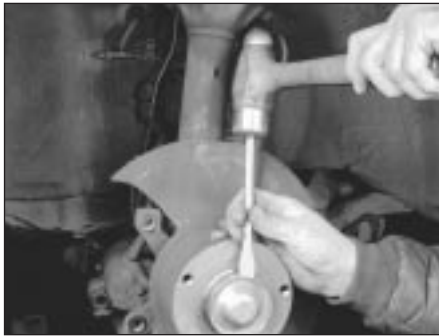
8.2 Using a hammer and chisel, knock out the dust cap in the centre of the hub
