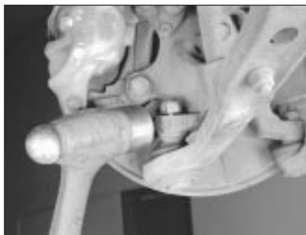
3.13b . . . give the steering knuckle a few sharp knocks with a hammer to release the balljoint stud from the strut housing, and remove the control arm
